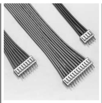
Measuring 2.0mm (.079") in pitch, 6.0mm (.236") in mounting height, and 3.25mm (.128") in thickness, this board-in connector meets the needs for high-density mounting on printed circuit boards efficiently and economically.
